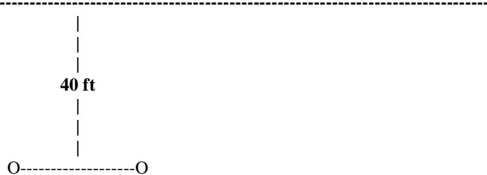
Procedure. Drive through the lane. Stop when the rear of the trailer is beyond the simulated gate. Back so that the trailer is perpendicular to and relatively centered on the real or simulated gate, within 6 feet of the gate.
